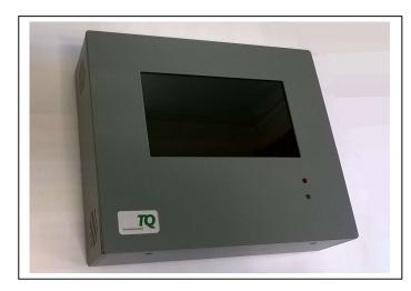
The TQ35 is a central alarm panel used to signal potential faults or alarms from multiple TQ32 remote alarm panels. Typically used in manned reception or security stations. Incorporates an internal buzzer and local mute to alert reception staff. Touchscreen display can quickly and easily be used to mute local sounders and identify specific locations in alarm.
